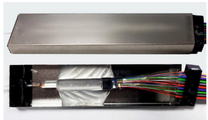
FIGURE 4 – Xyyyy-branded 1x32 splitter containing the insufficient amount of adhesive after testing in the environmental chamber.
